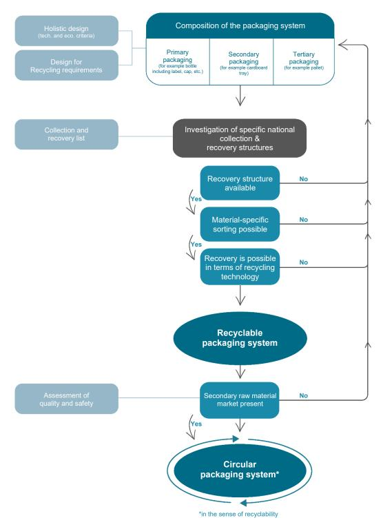
Figure 6 Steps in the design process
